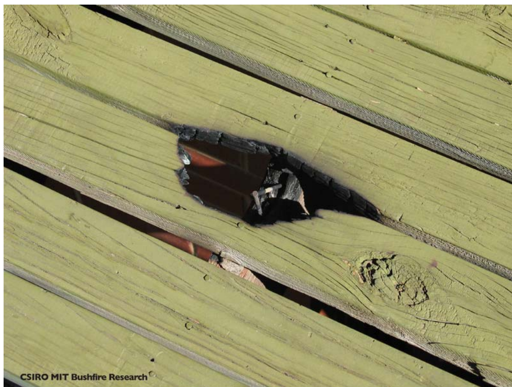
Figure 38. Ember attack on deck (with intervention)
