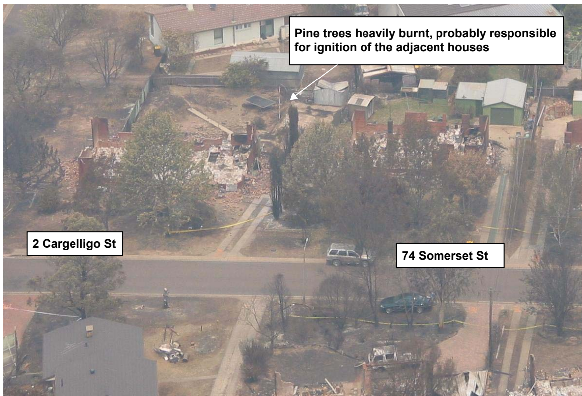
Figure 43. Pines fence responsible for ignition of 74 Somerset and 2 Cargelligo St
