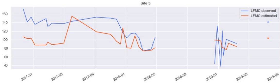
Figure 3. Line plot of average observed and estimate LFCM over time for different study sites. Note that there are data gaps in the LFCM observations as field data was not collected between 2018-04-27 and 2018-12-18 and in the satellite estimates mainly because of cloud coverage.
