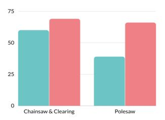
Figure 4: average heart rate (% max) during chainsaw field trials using medium chainsaws (blue, n=2) and large chainsaws (pink, n=2), for 12 and 6 minutes, respectively. polesaw use was observed once over 6 minutes (blue, n=2) and once over 14 minutes (pink, n=4).
