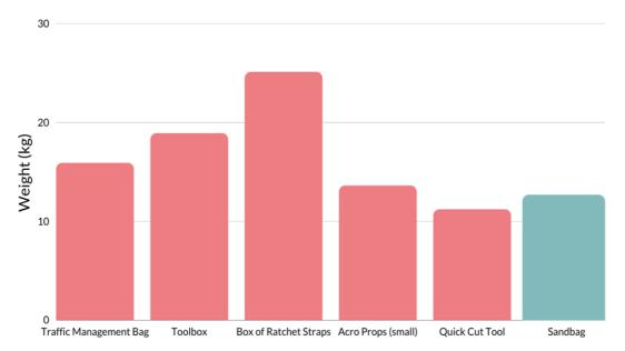
**Figure 14:** Typical mass of equipment required for a Storm Damage debris-clearing activity. Green = requires multiple lifts and carries.
