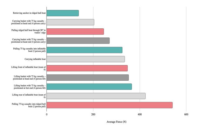
Figure 3: Average amount of force, in newtons, required to complete various boat operations tasks.
