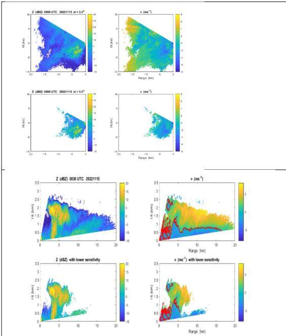
Figure 1: Panels show examples collected of horizontal (left) and vertical scans (right) around ash plumes on Nov 22, 2022. The top figures are the raw data while the lower panels are what the Furuno system would observe with its lower sensitivity.
