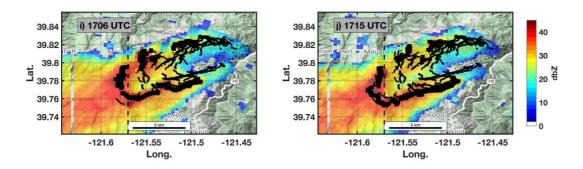
Figure 2. Two snapshots of Radar-derived fire progression during the early growth of the Camp Fire from 1500 to 1832 UTC. Each panel shows the radar reflectivity (shaded), the current fire perimeter estimates (solid black squares), previous perimeter points (small black squares), and a meridian indicating the eastern edge of the town of Paradise, CA. Taken from Lareau et al. (2022).
